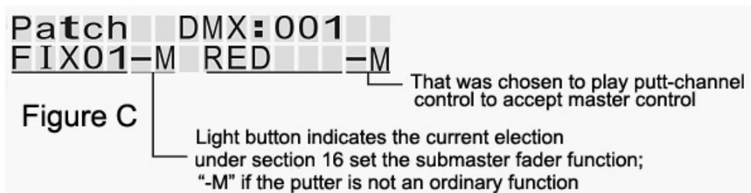
The first M indicates that the 16<sup>th</sup> slider for the current fixture is set as a master slider; If no M appeared, then, it is a normal slider. The second M indicates that the chosen slider channel is subject to the control of the master slider.
