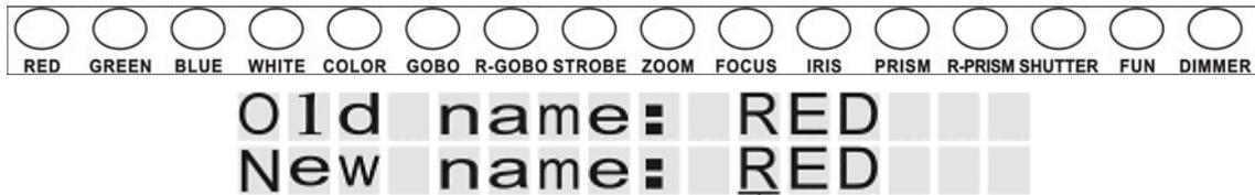
e. Move the joystick left or right to move the cursor; Move the joystick up or down to change the letter at the current position;
