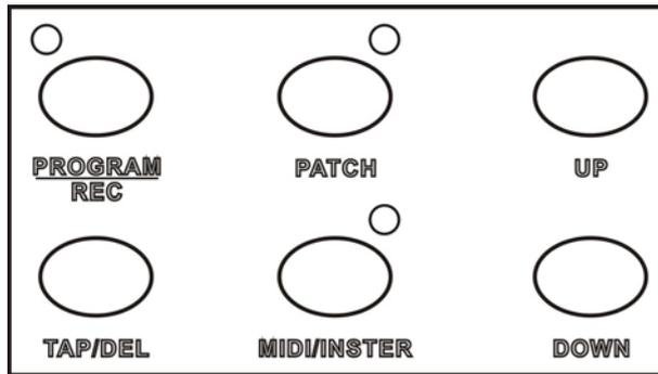
**PROGRAM/REC** is used to enter program mode or to confirm an operation. Press and hold it for three seconds, it will enter program mode; Press and hold again to exit. When in program mode, use it to record the current effect.
