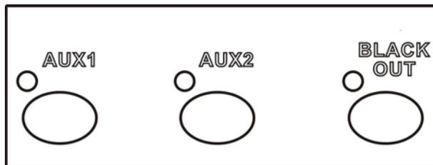
**AUX1** and **AUX2** are two additional buttons. One or several or all of the 256 channels can be assigned to the AUX buttons (press to set on/off). The button can also be programmed in scenes and chases.
