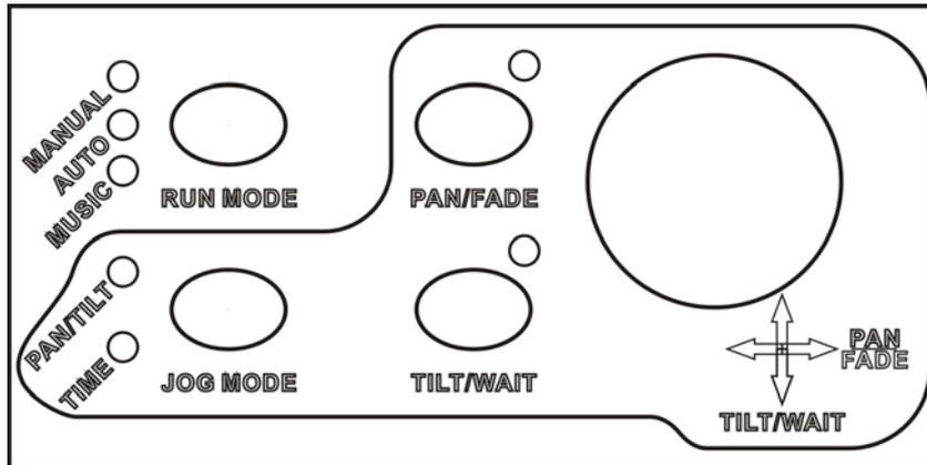
**JOG MODE** is the joystick function select button; When the PAN/TILT indicator turns on, the joystick to adjust the Pan/Tilt channels; when the TIME indicator turns on, the joystick is to adjust fade time and wait time of a chase;
