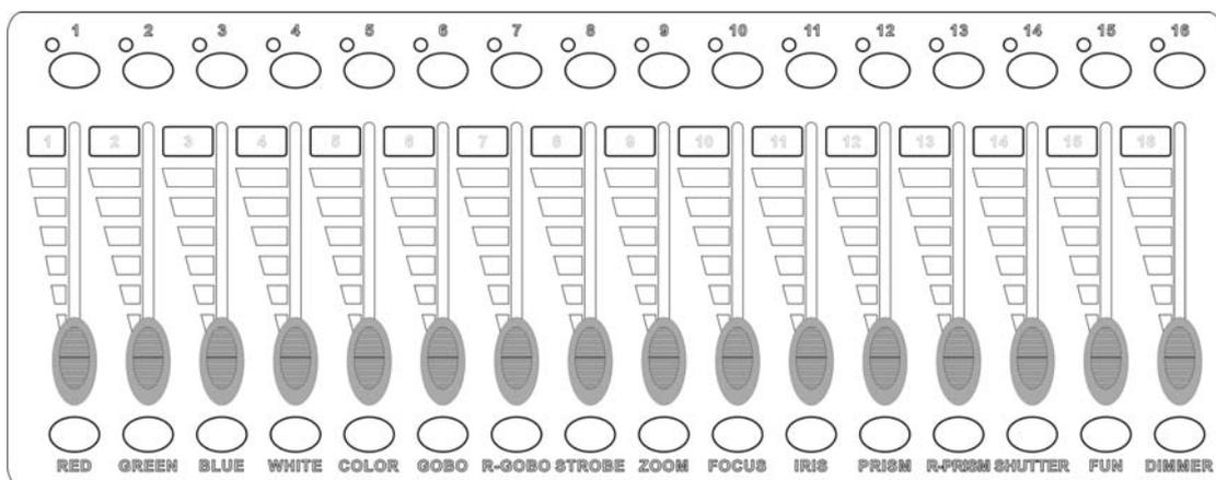
The fixture area consists of 16 fixture buttons in the upper row, 16 channel sliders in the middle row, and 16 press-control buttons in the bottom row. The fixture buttons are to select lighting fixtures. The channel sliders output the control data. Press the press-control button, the corresponding channel will output the value of 255. Once released, the output value will return to the slider value.
